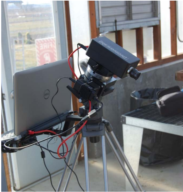
Figure 1. Tripod-mounted hyperspectral Imaging System and computer-controlled scanner.
