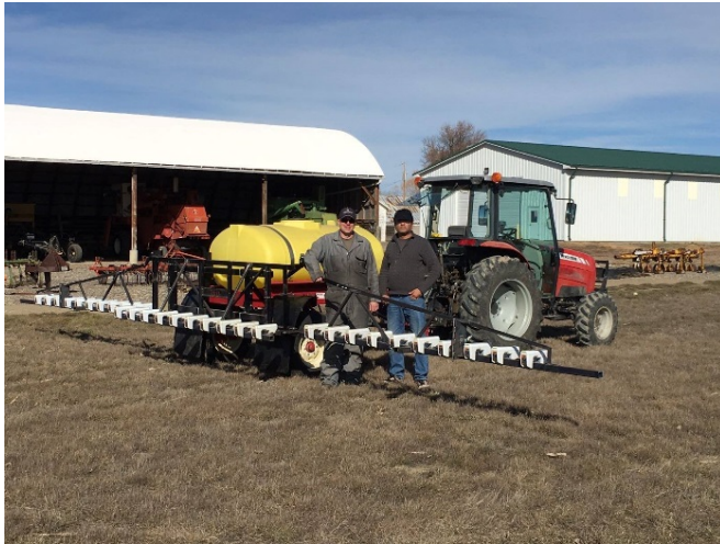
Figure 1: WeedSeeker sprayer with 30 LASC units for precision (site-specific spot spray) weed control in chemical fallow (2016).
