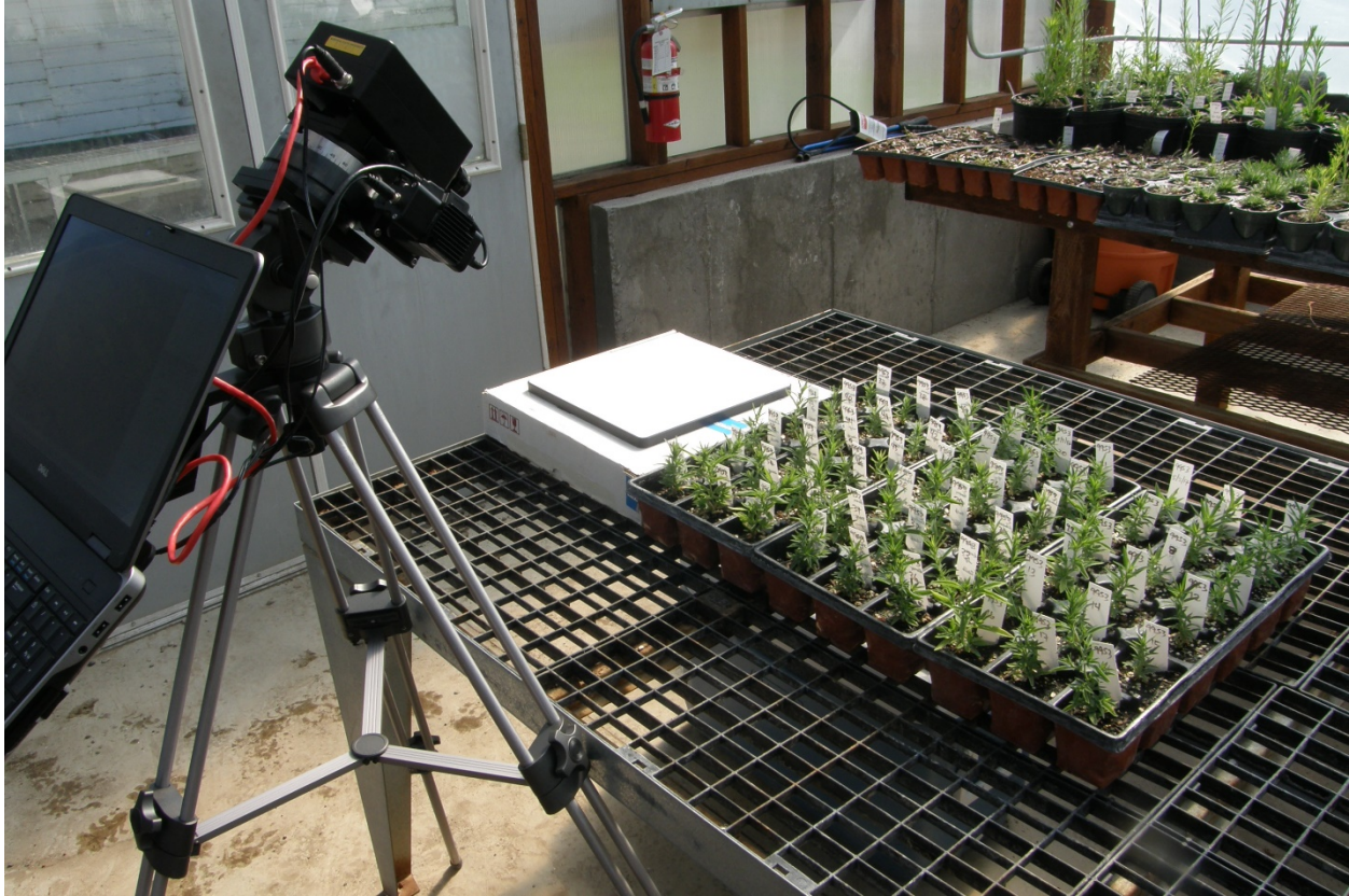
Figure 5. Tripod-mounted hyperspectral imager recording spectra of multiple plants at multiple growth phases.
